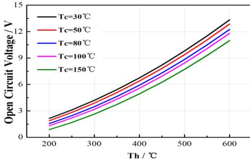
Open circuit voltage Vs  $T_h$  under various  $T_c$
