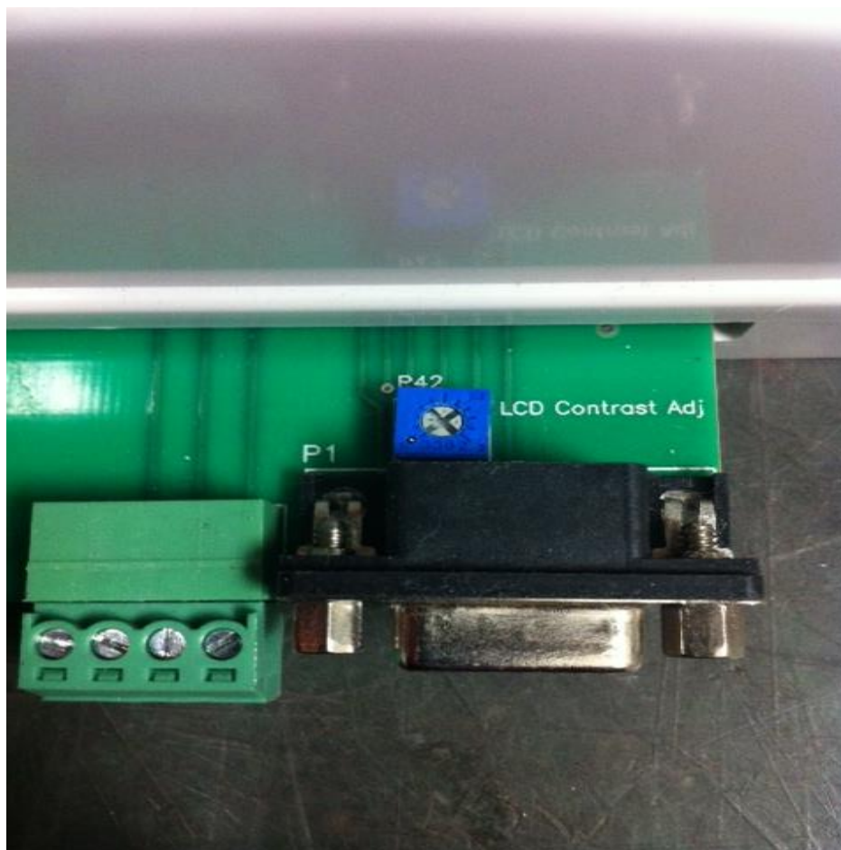
Fig.4 LCD Contrast Adjust panel when all DIP switches are in the down position to allow the contrast to be adjusted for seasonal ambient temperature variations.
